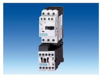
CONTACTOR, AC-3 5.5 KW/400 V, 1 NO, AC 230 V, 50/60 HZ, 3-POLE, SIZE S00, SCREW CONNECTION
