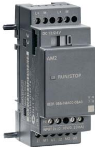
LOGO! AM2 EXPANSION MODULE, PU: DC 12/24V, 2 AI, 0 - 10V OR 0 - 20mA
