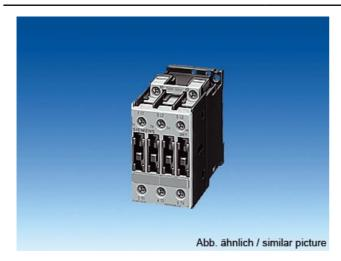
CONTACTOR, AC-3 5.5 KW/400 V, AC 230 V, 50 HZ, 3-POLE, SIZE S0, SCREW CONNECTION
